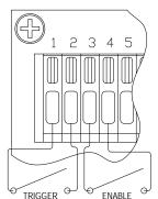
capability to trigger the system through telephone or computer control. Closure of the Trigger and Enable inputs will start one snow melting cycle, just as though the MANUAL ON button was pressed. Once the cycle is complete the sensor will revert to AUTOMATIC mode.
